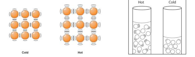
The higher the temperature the faster the molecules are moving.
